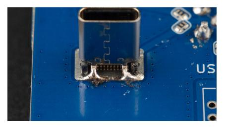
Solder both USB-C sockets, on one either half of the Output side of the board.
