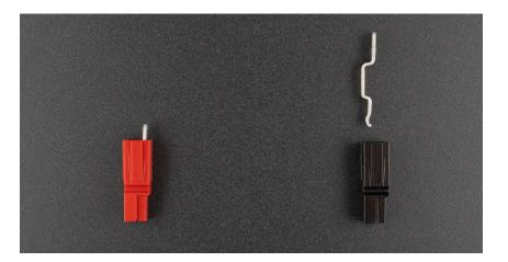
Inspect the metal tabs. Note that one end has a rounded bump on it. This is the mating surface of the connector. The other end is a straight tab, with little shoulders sticking out. This is the part that is soldered into the board.
