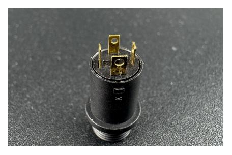
**Warning:** In early versions of the PCB (v3.1c) the pads on this outline were ... snug ... to put it kindly. You must insert the 3.5mm sockets with a fair bit of force.
