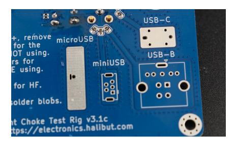
Note that the board has a large exposed pad onto which the microUSB socket will be soldered. (Same for the USB-C sockets, but we'll do those next.) The slot for the middle tab, and the hole of the plastic bump, can be seen. But otherwise, it's a very large area to solder to, to make it easier.
