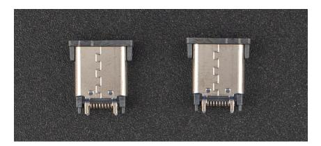
The two USB-C sockets are very similar to the microUSB socket described above. There are small plastic bumps on the bottom that have to line up with holes on the board for the socket to lay flush. There are four metal tabs on the corners of the connector that stick into the board a little bit. Again, these aren't long enough to solder from the bottom, so you must solder them from the top side.
