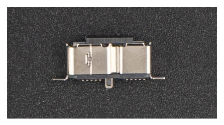
The microUSB socket has large metal tabs on either end of the connector that solder flush to the surface of the board, and a smaller metal tab in the middle that gets inserted into the board, like a normal through-hole part, except that it's not long enough to go all the way through to the other side. There is also a small plastic bump on the bottom of the part that has to line up with the hole in the board immediately adjacent to the slot that middle tab goes into.
