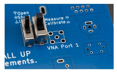
**Note:** SMA sockets have a lot of thermal mass, and will require more heat to solder than most throughhole components. If you have a higher wattage soldering iron, now is the time to break it out.
