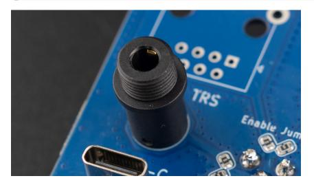
Make sure to solder both 3.5mm sockets, one on each side of the board. (The image is only showing one.)
