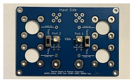
Do this for both SMA ports on the Input side of the board. It should look like this when you're done:
