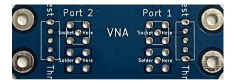
SMA sockets have a lot of thermal mass, and will require more heat to solder than most through-hole components. If you have a higher wattage soldering iron, now is the time to break it out.
