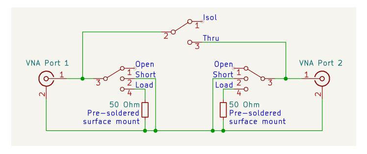
NOTE: When we talk about setting the "Open/Short/Load" switches, always set both switches the same.
