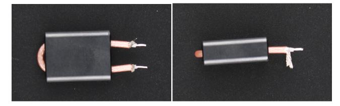
Insert the whole CMCC assembly (ferrite core, RG-316 in a U shape through the holes, ends of the RG-316 trimmed as described above) into the two holes on the phasing board labeled "CMCC." Make sure the twisted-sticking-out shields line up with the two exposed pads labeled "Shield" on the PCB.
