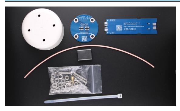
• Main Board: the circular board with four bolt holes around the edge
