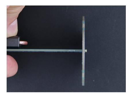
Once you're happy with the angle between the two boards, solder the rest of the pad joints, on both top and bottom.
