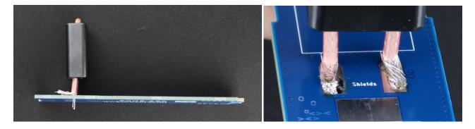
There should be about 3/8 to 1/2 inch (9 to 12mm) of exposed coax between the board and the ferrite core when you hold the ferrite core up away from the board -- enough to let the ferrite bend over against the board without crimping the coax. It should look like this:
