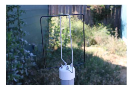
When forming the rectangles out of whatever material you're using, form the rectangles with the opening (the ends of the wire) in the center of the bottom.
