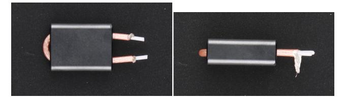
□ Cut the dielectric about 1/16in (1.6mm) (the thickness of the PCB) above the shield you've just twisted together, then strip it off exposing the center conductor. Err on the side of leaving a bit more dielectric rather than less; make the dielectric sticking out of the shield longer, not shorter. But get as close to the thickness of the PCB as possible.
