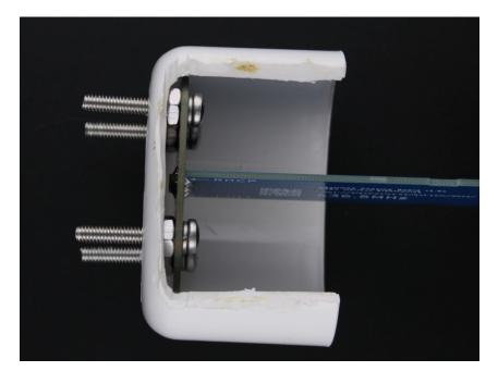
Add a rubber sealing washer onto each screw. They take a little force to work down the screw.
