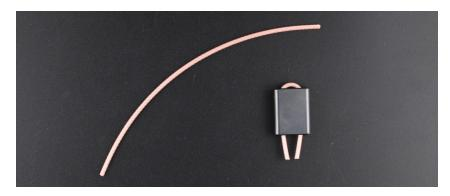
☐ Strip about 1/4 inch (8mm) of the outer jacket off both ends of RG-316.
