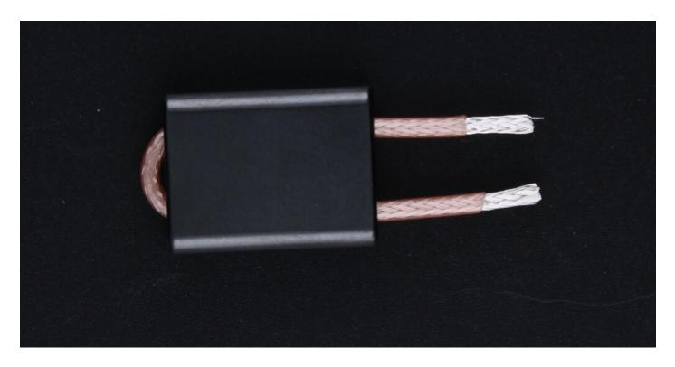
Unwrap the shield from the center dielectric, pull it all to one side, and twist it so that it sticks out at a 90° angle from the coax, out the wide side of the ferrite core. Do this so both ends of the coax's shields are sticking out the same side of the ferrite core. The shield around the coax should be as flat as possible; you're going to insert the dielectric through the PCB, so the shield is flush against the PCB, and the center pin sticks out the other side. It should look like this:
