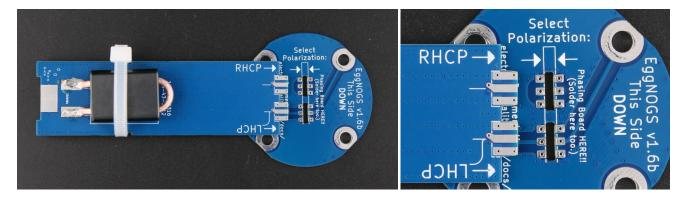
Pay attention to the main board's "This Side UP" and "This Side DOWN" text. The phasing board is inserted into the "This Side DOWN" side.
