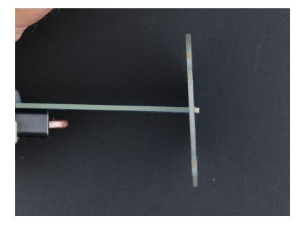
Warning: Do NOT try to just bend the solder joint to be perpendicular, you'll lift a pad off the board. Ask me how I know. If your board angle needs adjustment, use your soldering iron to reheat that one pad's solder joint and adjust. Now is the only opportunity you'll have to fix this.
