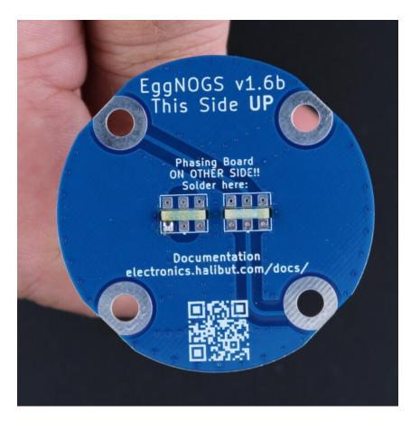
Inspect the angle between the two boards. If necessary, reheat that solder joint and adjust the angle to make the boards as perpendicular as possible. For example, I re-did this joint:
