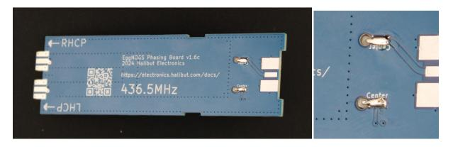
Solder the shields to the two large pads.
