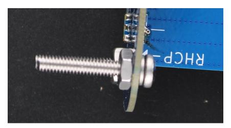
Insert the main board assembly (with all four screws on it) into the INSIDE of the PVC cap, with the screws protruding through the holes to the outside. The holes should line up cleanly with the screws.
